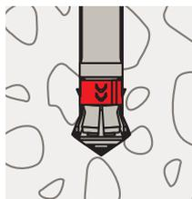
With **positive connection**, the anchor geometry adapts to the shape of the drill hole. The anchor makes maximum use of the load-bearing capacity of the substrate. There are no or only low expansion forces.
