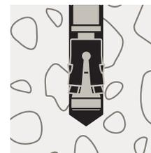
With **friction locking**, the expansion part of the anchor is pressed against the wall of the drill hole. The tensile forces are absorbed by friction.
