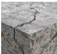
Cracked concrete C20/C25 to C50/C60
