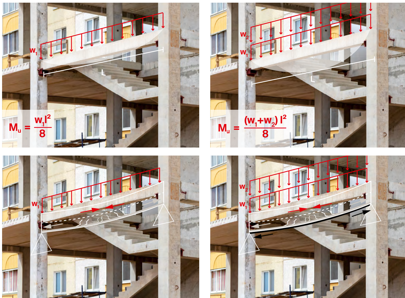
Fig. 4 – Left: unstrengthened beam, Right: flexural strengthened beam
