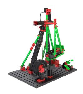
While building the model, make sure that the boat is just about in contact with the tyre. Then pivot the swing by hand and use the interface test to make sure that the Reed contact trips when the magnet on the swingboat passes the Reed contact.
