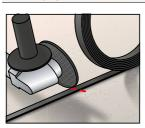
Be careful when loosening the packaging straps off the CFRP coil because the uncontrolled uncoiling can cause injuries. The coils are under tension when they are coiled. It is recommended to use a coiler for CFRP Laminates.
