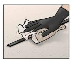
The surface of the fischer FRS-L-S NSM Laminate must be thoroughly cleaned using the fischer FRS-CA cleaning agent or acetone and a soft cloth.
