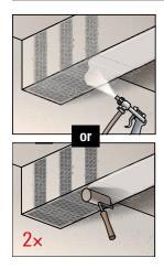
The application of the FRS-SF is carried out on the surface, onto which sand was previously hand-sprinkled.
