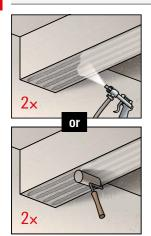
The application of the FRS-SF is carried out on the surface, onto which sand was previously hand-sprinkled.
