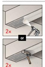
The UV Protection Coating FRS-SF can directly be applied on the surface of the externally bonded FRS-L-S and FRS-L-H CFRP Laminates (without prior sand sprinkling).
