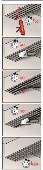
The FRS-CS 585 S should be injected into the concrete grooves.
