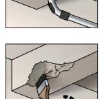
Apply the fischer FRS-BA Bonding Agent as a thin film layer on the concrete fracture surface using e.g. a brush. For the recommended thickness to be applied and detailed processing information please consult the Technical Data Sheet (TDS) of fischer FRS-BA.
