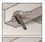
The damaged concrete fracture surface needs to be properly cleaned prior to the application of the concrete patching material or bonding agent. The concrete surface to be repaired or reprofiled must be dry, oil and dust free and the loose concrete parts must be removed. Tools such as steel brush, vacuum cleaner, compressed air might be used to clean the concrete surface.
