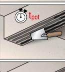
The FRS-CS is able to hold the own weight of the laminate in overhead applications without additional temporary fixing solutions. Excess FRS-CS can be removed and the surface smoothed with a trowel.
