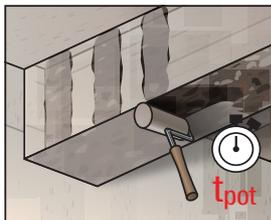
The saturating resin FRS-CF is applied with a roller on the concrete substrate. Take care to adjust the consumption of FRS-CF to the roughness of the surface.
