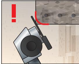
The sharp concrete edges must be rounded to corner radius of > 13 mm according to ACI 440.2R.
