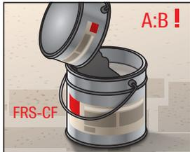
Add component B to component A and mix it (handheld agitator) for 3 minutes with 300 rpm without air bubbles until a homogeneous and uniform gray tone is achieved.
