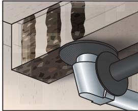
The concrete surface, where the strengthening products will be applied must be roughened up by means of one of the following techniques:
