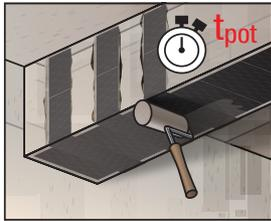
After the last CF Fabric layer, the last layer should be coated with  $0.5\text{--}0.7\text{ kg/m}^2$  FRS-CF.
