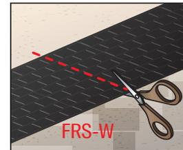
The Carbon Fiber Fabrics FRS-W U300 & FRS-W U600 shall be completely dry, free of oil and dust and the surface on the entire length must be checked for visible damage such as undulations.
