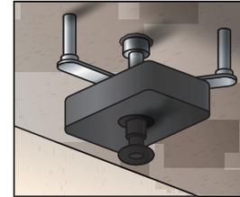
Prior to application of the CF Fabrics, the suitability of the concrete surface must be verified through concrete pull-off tests. The concrete surface tensile strength is to be determined using a concrete pull-off device. If concrete repair works were performed, the surface tensile strength has to be determined on the reprofiled concrete surface.
