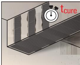
The CF Fabrics does not require additional supportive temporary fixing solutions during the curing process.
