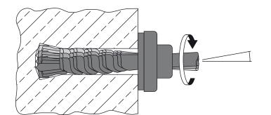
One operation: cylindrical drilling – swivel undercut.
