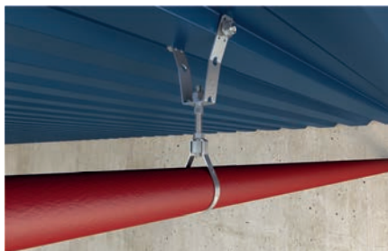
Sprinkler pipe installation to trapezoidal metal sheet
