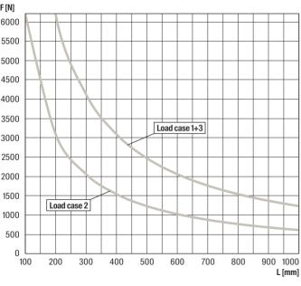
For the load curves, the permissible steel strain  $\delta_{adm.}$  = 160 N/mm and the maximum deflection under load L/150 are not exceeded. Load values of the cantilever arms under consideration of the load capacity of the base plate. Fixings and screw fastenings must be calculated accordingly. The load curves are valid for all material thicknesses of the FCA brackets.
