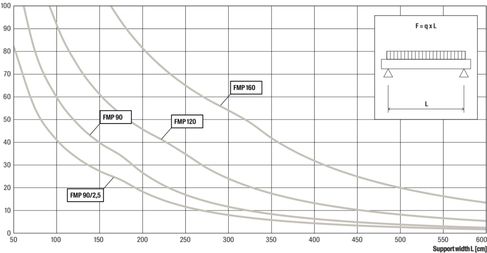
\*\* The permissible stress is calculated acc. EN 1993;  $\sigma_{rec} = f_{yk} / (\gamma_L \cdot \gamma_{MO})$  with  $\gamma_L = 1,4$  and  $\gamma_{MO} = 1,0$ . Lower value of permissible stress (shear, bending or combined) or max. deflection ( $L/200$ ) is decisive
