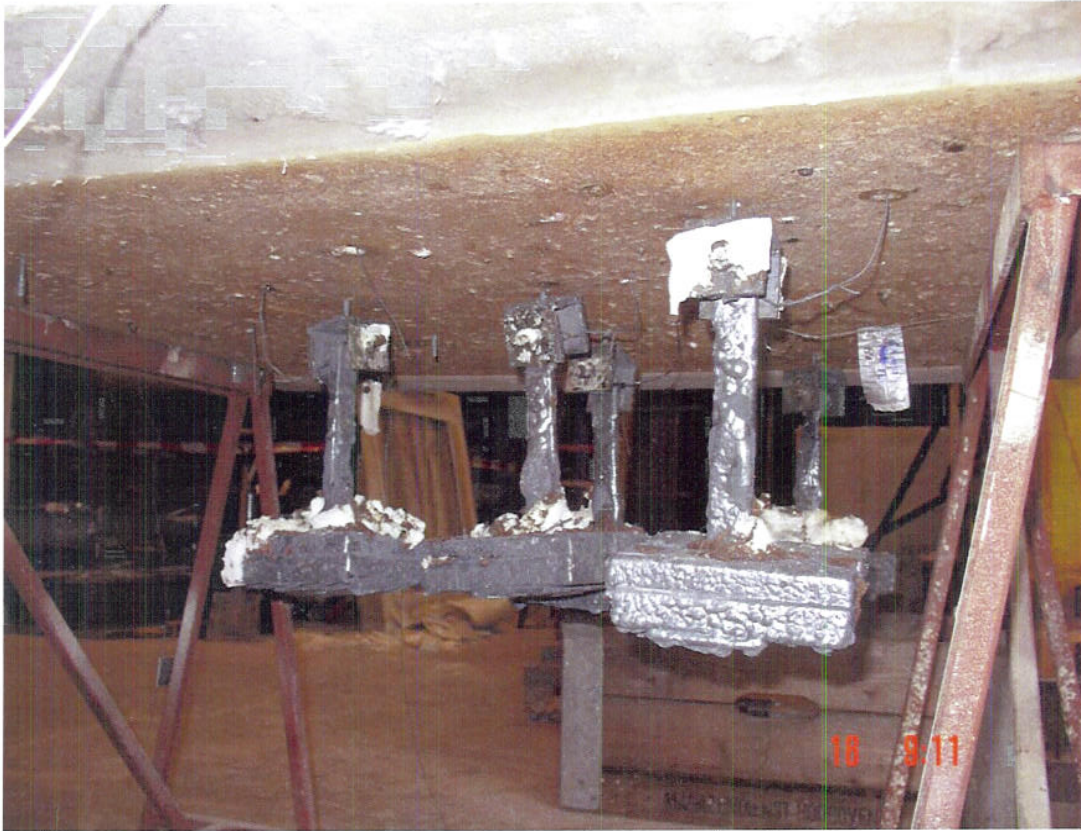
Photo 3 : view of the test specimen after heating and cooling down
