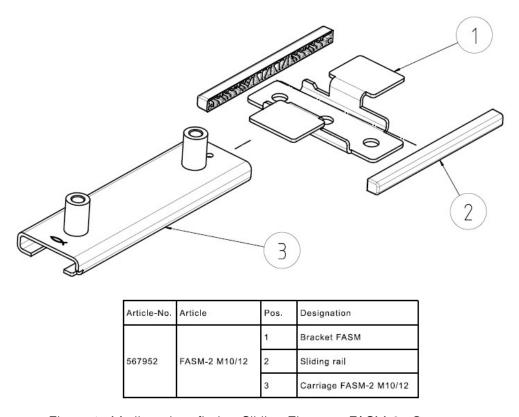
Figure 1: Medium-duty fischer Sliding Elements FASM-2: Geometry
