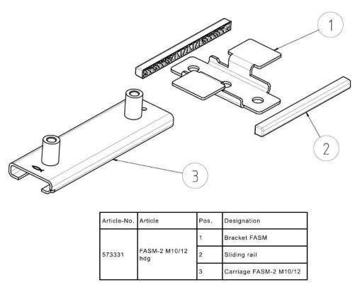
Figure 2: Medium-duty fischer Sliding Elements FASM-2 HDG: Geometry
