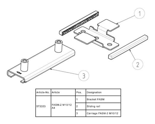
Figure 3: Medium-duty fischer Sliding Elements FASM-2 A4: Geometry
