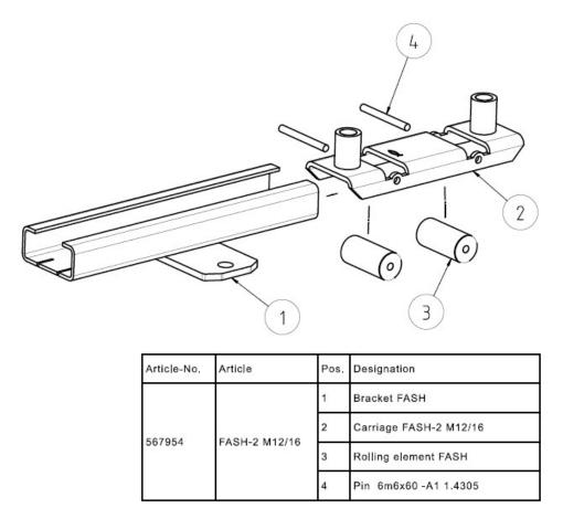
Figure 4: Heavy-duty fischer Sliding Elements FASH-2: Geometry
