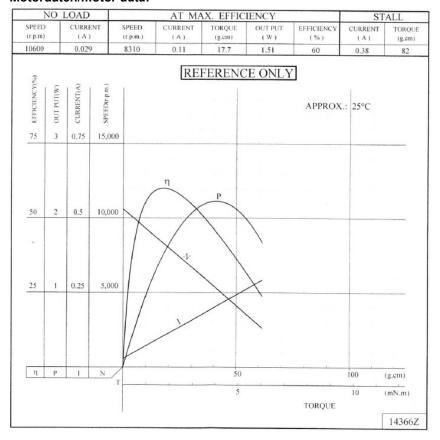
Nennspannung Motor/rated voltage motor: 24V DC
