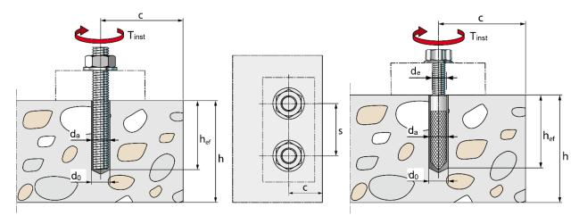
THREADED ROD / REINFORCING BAR
