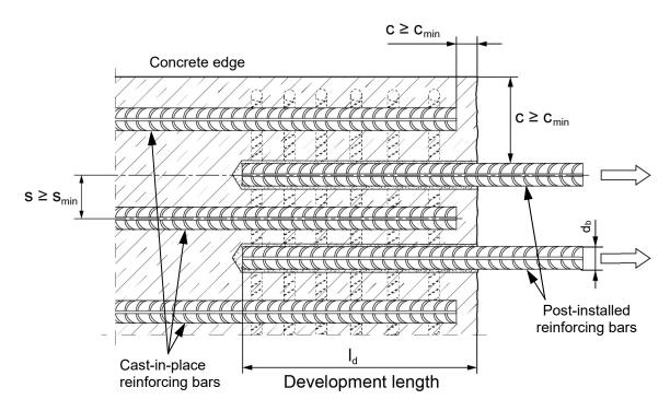
FIGURE 2—GENERAL INSTALLATION PARAMETERS FOR POST-INSTALLED REINFORCING BARS
