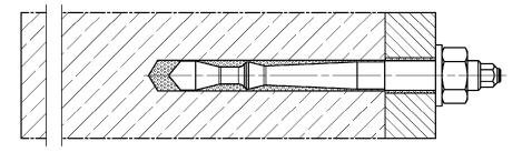
**Pre-positioned or push through installation** with subsequently injected fischer filling disc (annular gap filled with mortar)
