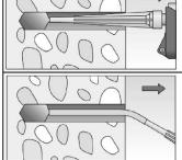
Fill approximately 2/3 of the drill hole with mortar. Always begin from the bottom of the hole and avoid bubbles
