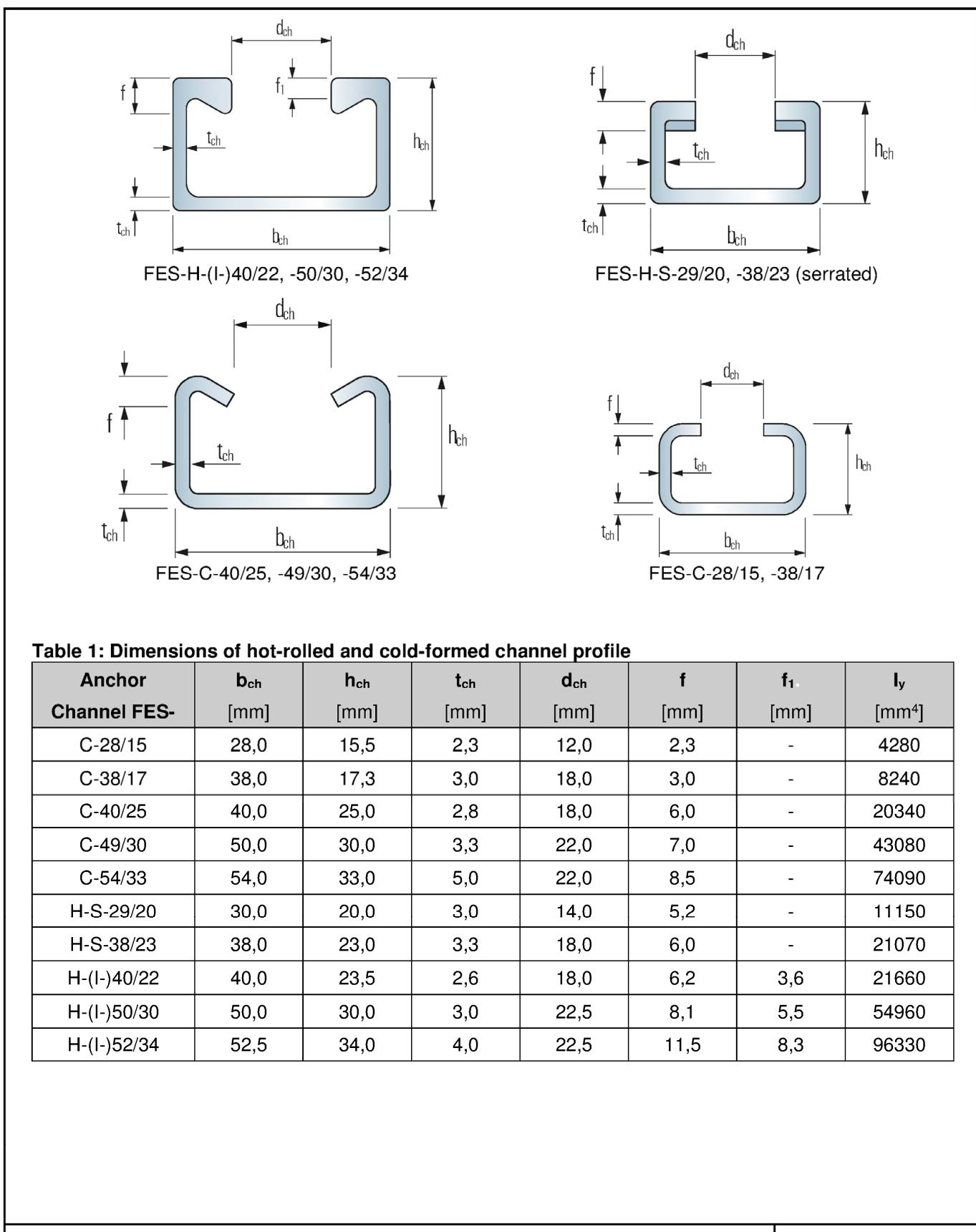
**Table 1: Dimensions of hot-rolled and cold-formed channel profile**
