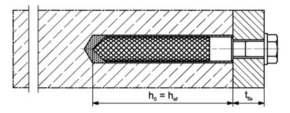
Pre-positioned installation with subsequently pressed filling disk (annular gap filled with mortar)
