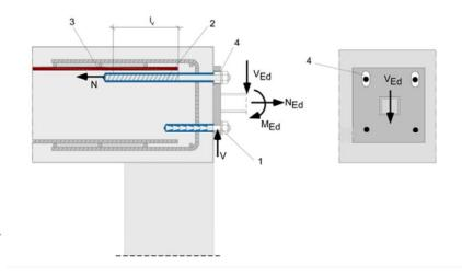
The required transverse reinforcement acc. to EN 1992-1-1:2004+AC:2010 is not shown in the figures. **The fischer rebar anchor may be only used for axial tensile force.** The tensile force must transferred by lap to the existing reinforcement of the building. The transfer of the shear force has to be ensured by suitable measure, e.g. by means of shear force or anchors with European Technical Assessment (ETA).
