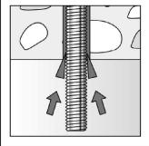
For overhead installation, support the rebar / fischer rebar anchor and secure it from falling till mortar started to harden, e.g. using wedges.
