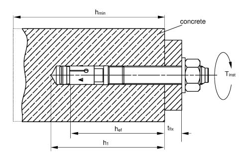
$\begin{array}{lll} h_{\text{ef}} & = & \text{Effective embedment depth} \\ t_{\text{fix}} & = & \text{Thickness of the fixture} \end{array}$
