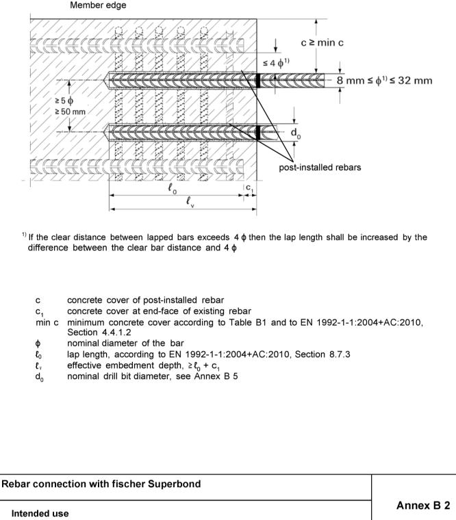
General construction rules for post-installed rebars
