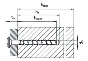
d0=nominal drill bit diamterhnom=nominal anchorage depthh1=depth of the drill hole
