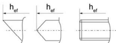
Alternative head geometry threaded rod FIS A and RGM
