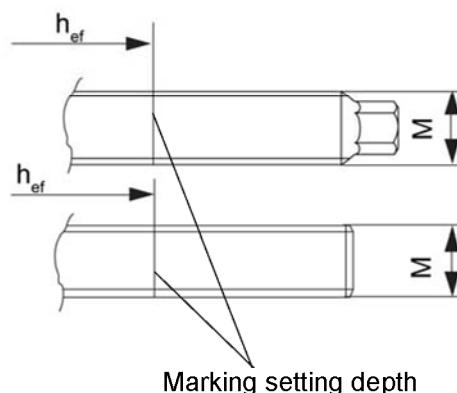
Alternative point geometry threaded rod RGM
