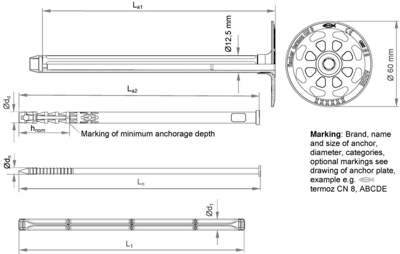
**Marking:** Brand, name and size of anchor, diameter, categories, optional markings see drawing of anchor plate, example e.g. termoz CN 8, ABCDEF
