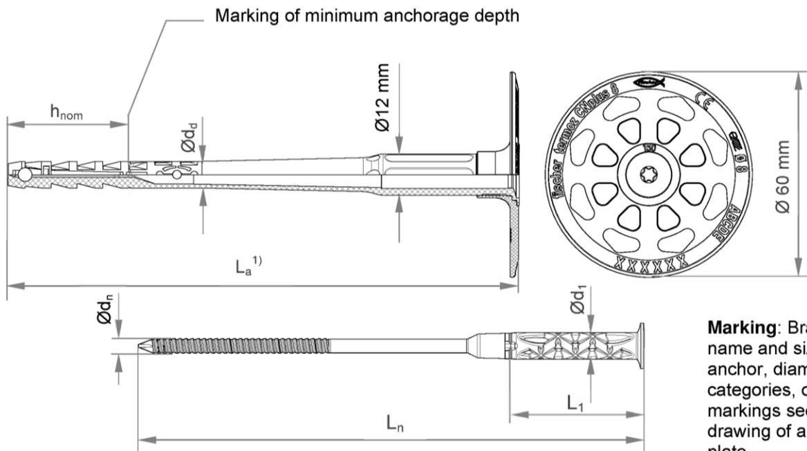
**Marking:** Brand, name and size of anchor, diameter, categories, optional markings see drawing of anchor plate, example e.g.
