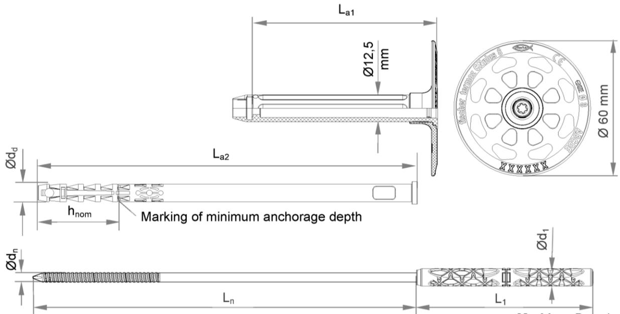
**Marking:** Brand, name and size of anchor, diameter, categories, optional markings see drawing of anchor plate, example e.g.
