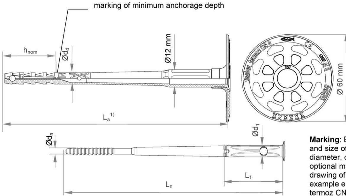
**Marking:** Brand, name and size of anchor, diameter, categories, optional markings see drawing of anchor plate, example e.g. termoz CN 8 ABCDEF
