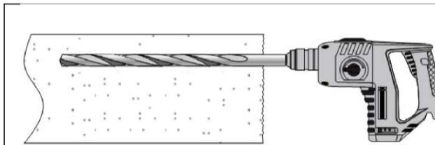
Drill hole to the required embedment depth using a hammer-drill with carbide drill bit set in rotation hammer mode, a pneumatic drill or a diamond drill in drilling mode.
