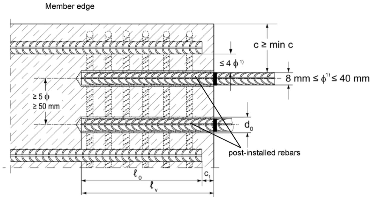
¹) If the clear distance between lapped bars exceeds  $4 \phi$  then the lap length shall be increased by the difference between the clear bar distance and  $4 \phi$
