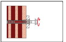
4. The screw is screwed-in until the head of the screw touches the sleeve. The anchor is correctly installed, if the head of the screw fits tight on the surface and nor the anchor sleeve neither the screw cannot be turned-in any further.
