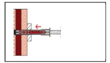
Insert anchor (screw and sleeve) by using a hammer until the collar of the plastic sleeve is flush with the surface of the fixture.
