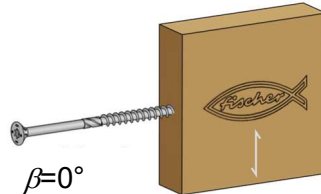
Figure D6.1: Screw arrangement in the narrow surface of OSB (figure not to scale)
