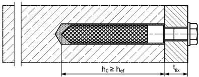
Pre-positioned installation with subsequently injected fischer filling disc (annular gap filled with mortar)
