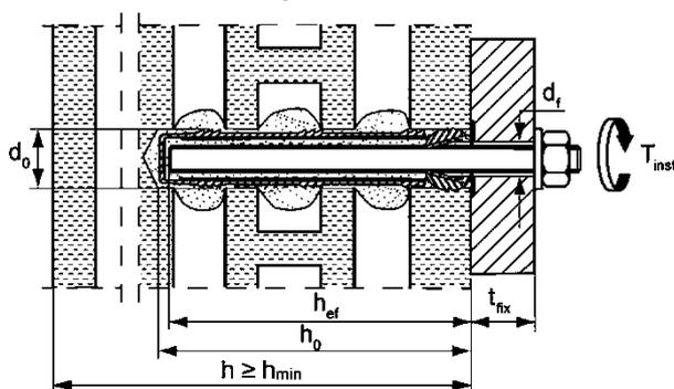
Internal threaded anchor with perforated sleeve
