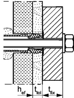
**Size of the perforated sleeve:** FIS H 12x50 K      FIS H 16x85 K      FIS H 20x85 K      FIS H 20x200 K
