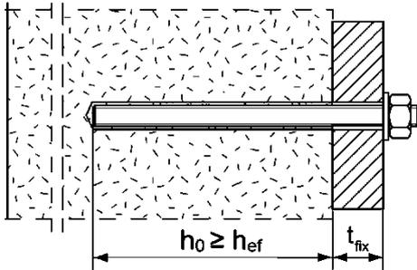
**Push through installation: Annular gap filled with mortar**
