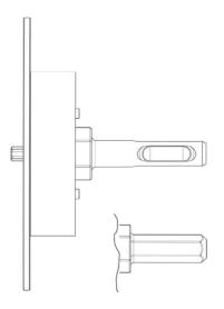
1) Alternatively, it is possible to mill the insulation material with a standard, market-available milling tool.
