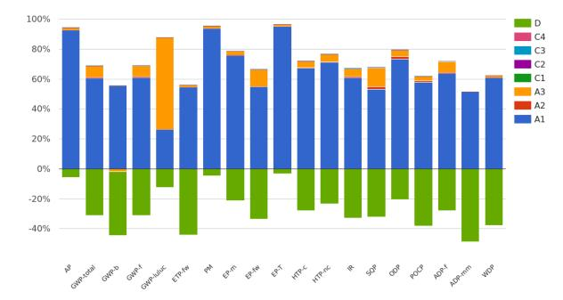
As can be seen in the graph, the raw material supply (module A1) has the highest impact for most environmental impact categories. Furthermore, for the benefits and loads beyond the product system boundaries (module D) the benefits (negative values) dominate over the loads (positive values) in most of the environmental impact categories.
