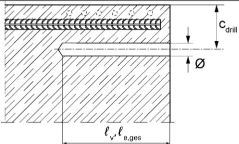
Measure and control concrete cover  $c$
