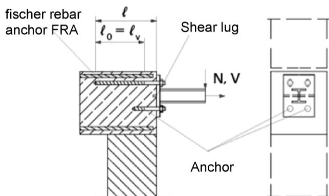
**Figure A8:** Lap of the anchoring of cantilevered buildings.
