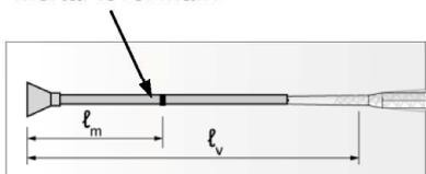
Mark the required mortar level  $l_m$  and embedment depth  $l_v$  resp.  $l_{e,ges}$  with tape or marker on the injection extension tube.
