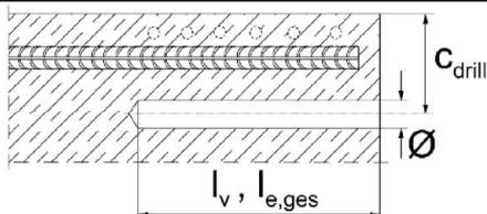
Measure and control concrete cover  $c$
