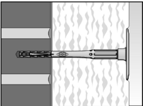
4. Correctly installed anchor.
