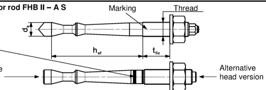
**Marking:** work symbol, size of anchor, setting depth. e.g.:
