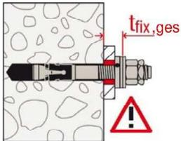
10: Correctly installed fastener
