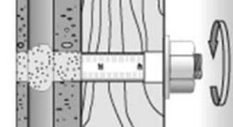
Tighten the hexagon nut.<br>$T_{inst,max}$ see Table B1.4                                                                          |
