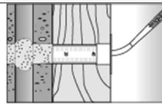
Fill the sleeve with mortar beginning from the bottom of the drill hole. <sup>1)</sup> For deep drill holes use an extension tube. |
