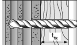
Drill the hole through the fixture. Depth of drill hole ( $h_0+t_{fix}$ ) and drill hole diameter see Table B1.4                     |
