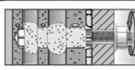
Tighten the hexagon nut.<br>$T_{inst,max}$ see Table B1.3                                              |
