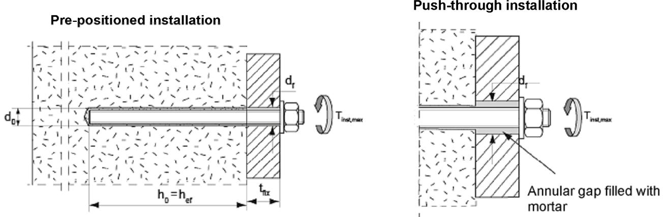
Internal threaded anchors FIS E without perforated sleeve FIS H K; Installation in solid brick masonry and aerated concrete
