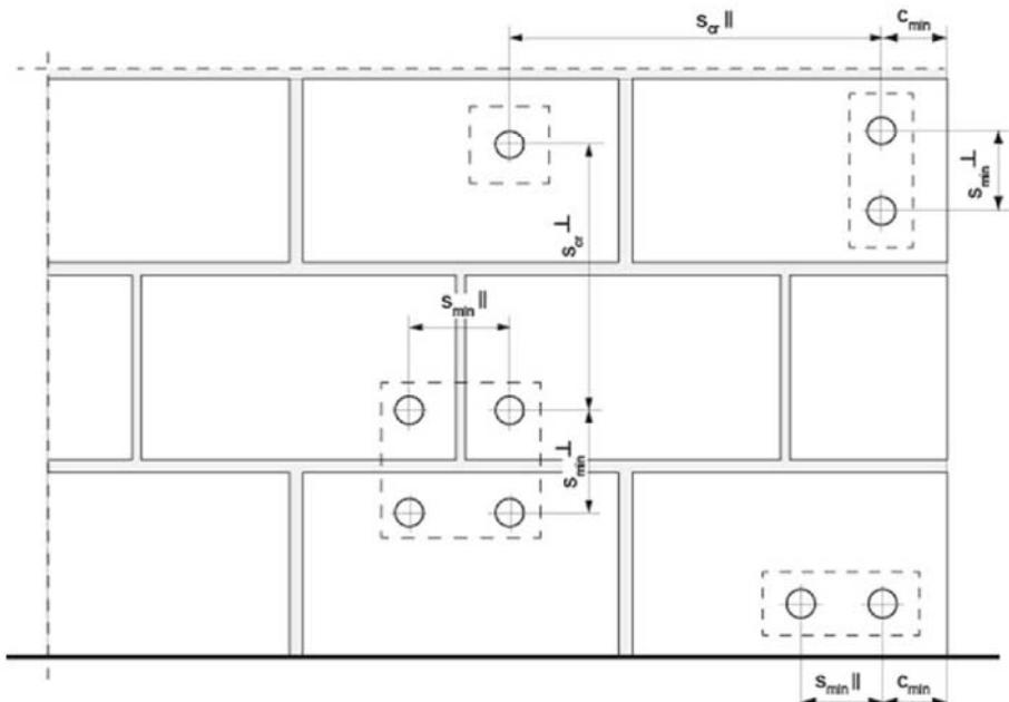
$s_{min \parallel}$  = Minimum spacing anchor group parallel to bed joint
