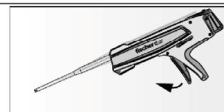
After injecting, release the dispenser. This will prevent further mortar discharge from the mixing nozzle.
