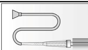
Assemble mixing nozzle FIS MR Plus or FIS UMR, extension tube and appropriate injection adapter (see table B 6.2)
