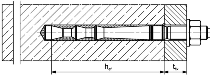
Push through installation not with mortar capsule (annular gap filled with mortar)
