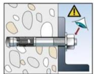
4: check setting position: Visible one turn of a thread
