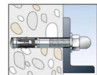
7: Installed fastener
