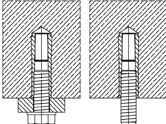
**Intended use in precast pre-stressed hollow concrete slabs ( $w/e \leq 4,2$ ) with a flange thickness  $d_b \geq 35 \text{ mm}$  (or 30 mm → see Annex C2) and only for  $h_{ef} = 25 \text{ mm}$**
