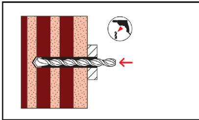
1. Drill the bore hole as per Table B2.1 using the drilling method described in the corresponding Annex C.
