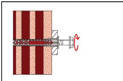
4. The screw is screwed-in until the head of the screw touches the sleeve. The anchor is correctly installed, if the head of the screw fits tight on the surface and nor the anchor sleeve neither the screw cannot be turned-in any further.
