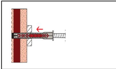
3. Insert anchor (screw and sleeve) by using a hammer until the collar of the plastic sleeve is flush with the surface of the fixture.
