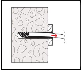
For application in hollow or perforated bricks, removal of bore dust is not necessary.
