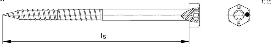
1) Additional marking for the special screw, stainless steel version: e.g. "A4" or "R" or "A2".
