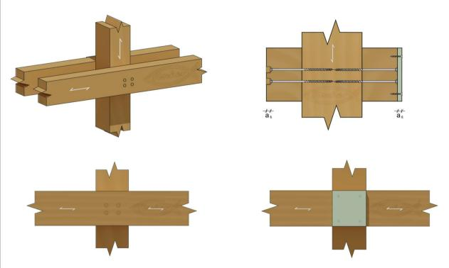
Figure J2.1: Fire design for protected screws – laterally loaded (figures not to scale)
