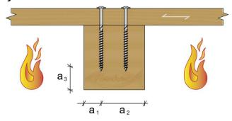
Figure J4.1: Fire design for axially loaded screws (figure not to scale)
