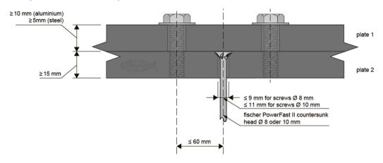
Figure L1.1: Screw head supporting plate for fischer PowerFast II screws (figure not to scale)
