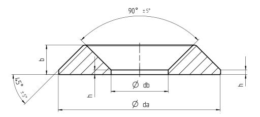
Washer for Power-Fast and construction screws
