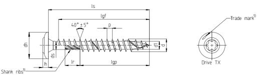
Power-Fast wood construction screw - Flange head with full- or partial thread
