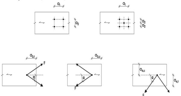
Definition of spacing, end and edge distances in the edge surface unless otherwise specified in the technical specification (ETA or hEN) for the cross laminated timber.
