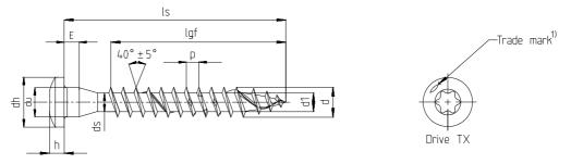
Power-Fast self-drilling screw - Wood connector screw with full thread
