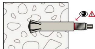
**5.:** The anchor is correctly expanded if the colour marking on the thread of the tapered bolt is visible or the gap  $u$  between conical bolt with internal thread and expansion sleeve (FZA I) is fulfilled. When using the FZA 12x40 ST the knurling on the sleeve is flush or below the concrete surface.
