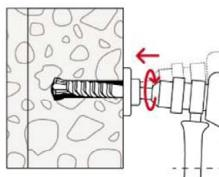
**2.:** Once the FZUB depth stop meets the concrete, create the drill hole undercut by making circular swiveling movements with the hammer drill while the hammer mechanism is engaged. Press the hammer drill firmly against the anchor base: 1 - 2 swiveling movements are sufficient for  $\varnothing 14\text{ mm}$ , with 3 - 5 movements for  $\varnothing 18\text{ mm}$  and  $\varnothing 22\text{ mm}$ .
