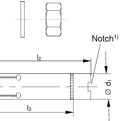
**Table A5.1:** Dimensions through bolt anchor FZA D [mm]
