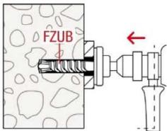
1.: Create a drill hole through the installation object perpendicular to the surface of the anchor base with a hammer drill, using the corresponding Zykron universal drill bit FZUB. The required drill depth is reached once the FZUB depth stop meets the fixture.
