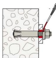
**Optional:** The gap between bolt and fixture may be filled with mortar (compressive strength  $\geq 50\text{ N/mm}^2$  e.g. FIS SB) after step 6 (for eliminating the annular gap). The filling disc is additional to the standard washer. The thickness of the filling disc must be considered for definition of  $t_{fix}$ . Countersunk of the filling disc in direction to the anchor plate.
