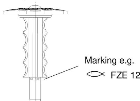
Centring pin for setting tool FZE Plus:
