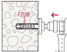
**1.:** The drill hole must be drilled at right angles ( $+/- 5^\circ$ ) to the surface of the anchor base with a hammer drill using the corresponding ZYKON FZUB drill bit. The required drilling depth is reached when the depth stop of the FZUB is in contact with the concrete.
