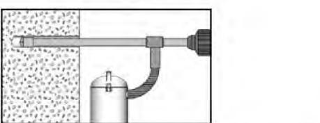
Drill the hole to the required embedment depth using a hammer drill with hollow drill bit in rotation hammer mode.
