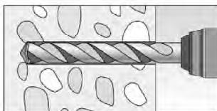
Drill the hole to the required embedment depth using a hammer drill with carbide drill bit set in rotation hammer mode or a pneumatic drill.
