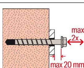
In the case of adjustment, the screw may be unscrewed by a maximum of  $L_{adj} = 20\text{mm}$ .
