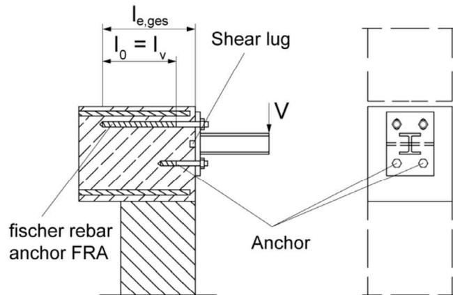
The required transverse reinforcement acc. to EN 1992-1-1:2004+AC:2010 is not shown in the figures. **The fischer rebar anchor FRA may be only used for axial tensile force.** The tensile force must be transferred by lap to the existing reinforcement of the building. The transfer of the shear force has to be ensured by suitable measure, e.g. by means of shear force or anchors with European Technical Assessment (ETA)
