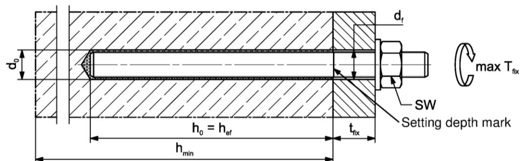
Commercial standard threaded rods, washers and hexagon nuts may also be used if the following requirements are fulfilled
